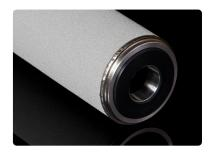
P is a robust material manufactured from sinterbonded metal powders. Primarily produced in 316L grade for use in temperatures up to 420°C (788°F), depending on process conditions, and offering resistance to most chemicals, P media can also be produced in other grades of stainless steel and alloys such as Inconel®, Hastelloy® and Monel®.
